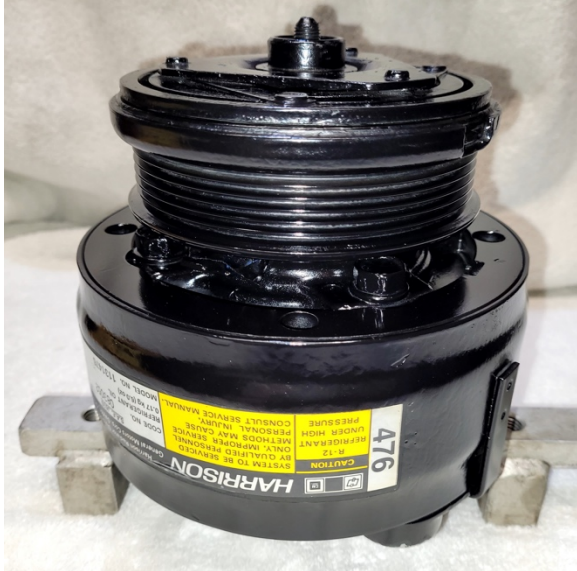
Rebuilt compressor, ready to install.
